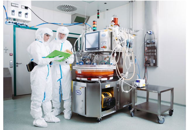
Exemplary image of an iCELLis 500 reactor empowered with Lucillus® at IDT in Braunschweig.
